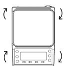
At the time of shipment, the adjusters provided at the four corners of the bottom are locked. Turn them in the direction shown in the figure on the left to loosen them.
