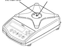
Place the pan base by aligning it to the projections provided on the main unit and then fix it by turning the screws using a tool such as a coin.
