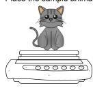
When weight variations fit within the set range, the value is held. Holding the readout is reported with "" shown in the display.
