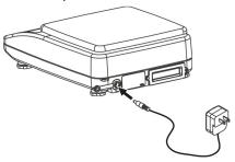
Connect the jack provided on the rear of the main unit to a power receptacle using the AC adapter.
